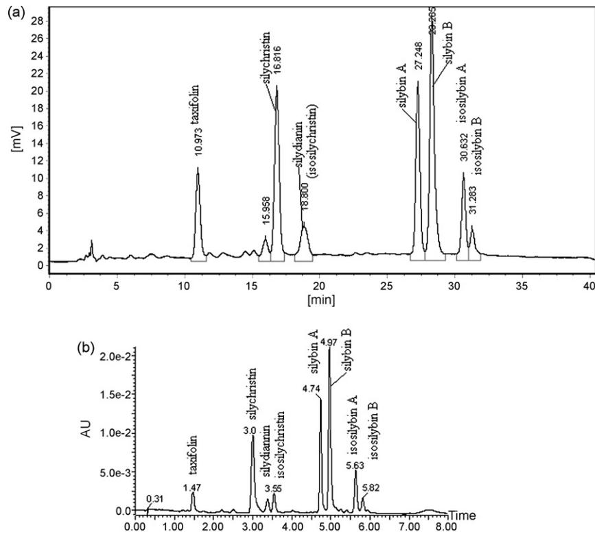
Fig. 2. Comparison of chromatograms of silymarin extract by (a) HPLC and (b) UPLC at wavelength 288 nm.
