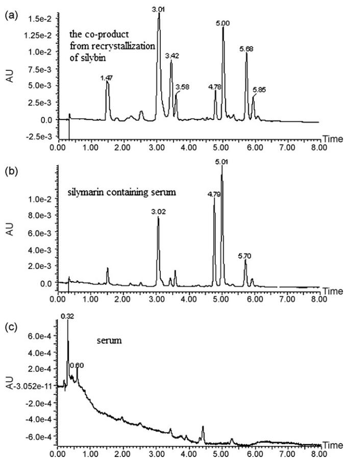
**Fig. 3.** Chromatograms of all active compounds in co-product of silybin recrystallization and silymarin containing serum by UPLC: (a) co-product of silybin recrystallization, (b) silymarin containing serum and (c) blank serum at wavelength 288 nm.
